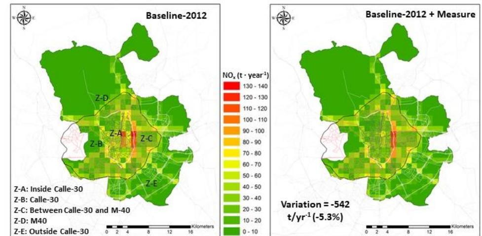
Figure 2. Example of the quantification of annual emissions of NO<sub>x</sub> of a measure applicable to road traffic in the Municipality of Madrid
