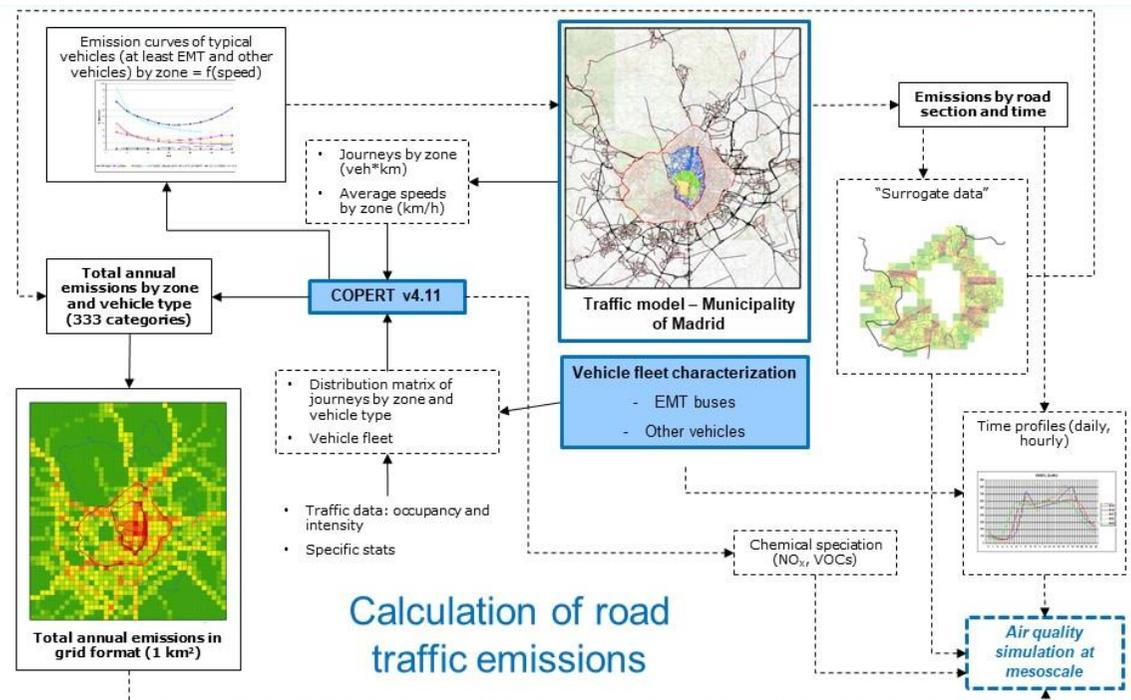
Figure 1. Diagram showing of the methodology used to estimate emissions from road traffic in Madrid and preparation for its use in the air quality simulation system at mesoscale
